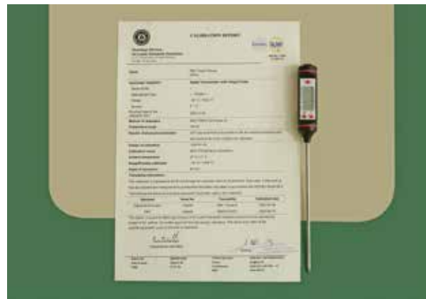
Photo 28: Probe thermometer with calibration report issued by a conformity assessment body
