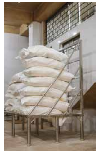
Photo 17: Temporary storage of wheat flour at a bakery on a stainless-steel rack that is 15 cm above the ground
